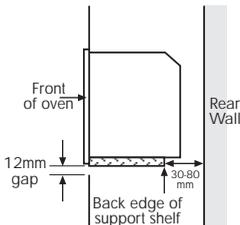
The appliance is designed to fit into a standard 600mm wide housing unit, with minimum internal dimensions as shown.
